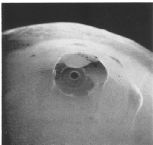
Figure 1 Scanning electron micrograph of the three {211} type facets observed on \langle 111 \rangle axis Y_3Al_5O_{12} single crystals ( \times 16 ).
